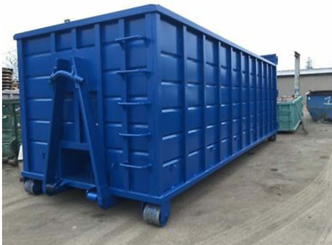
Figure 1. Similar design of roll-on roll-off storage container to those proposed (Courtesy of Machinery Line Ltd)
