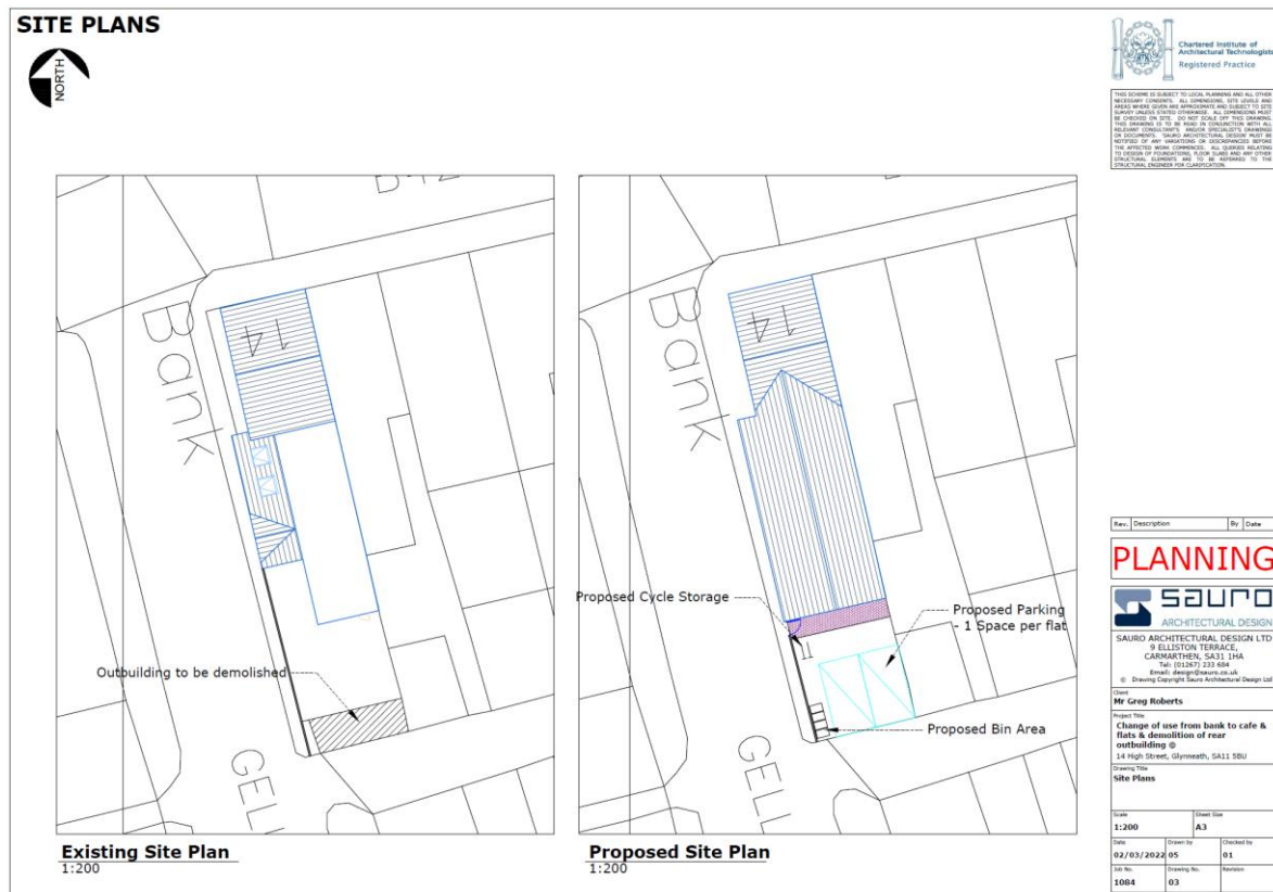
Figure 3: Site plans (provided by the architect)
