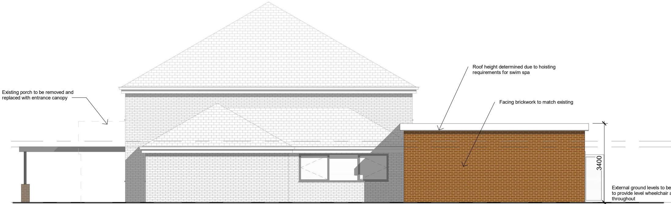
PROPOSED EAST ELEVATION 1 : 100
