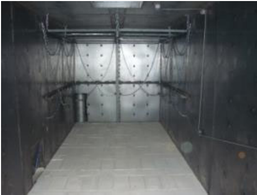
Inner view of the burn room with a floor made of fire resistant bricks and flexible smoke barrier for the regulation of the smoke entrance into the observation room
