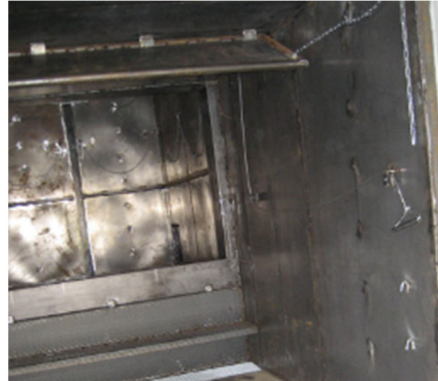
Inner view of the burn room with a floor made of fire resistant bricks and flexible smoke barrier for the regulation of the smoke entrance into the observation room
