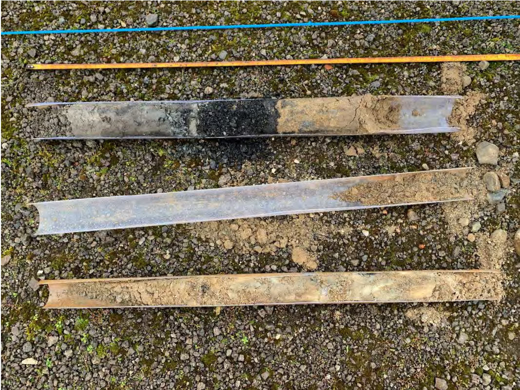
Photograph 5: Materials recovered from WS01, 0.0 – 3.0mbgl.
