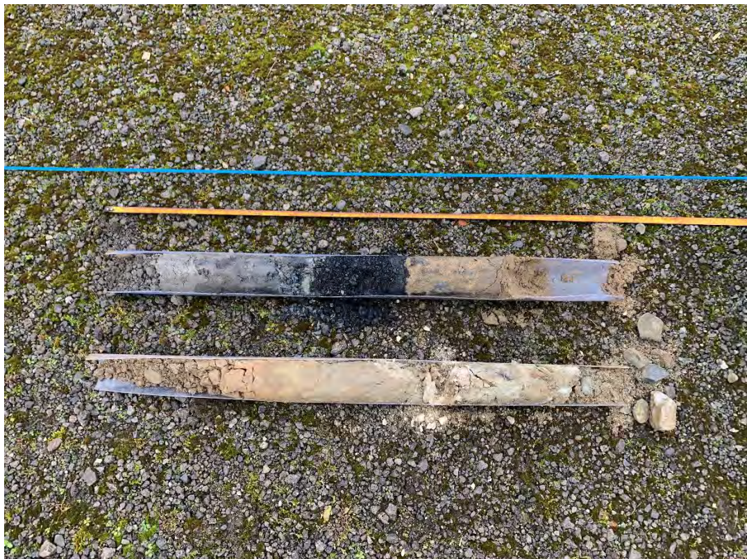
Photograph 4: Materials recovered WS01, 0.0 – 2.0mbgl.
