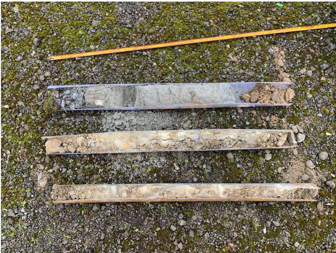
Photograph 6: Materials recovered from WS02, 0.0 – 3.0mbgl.
