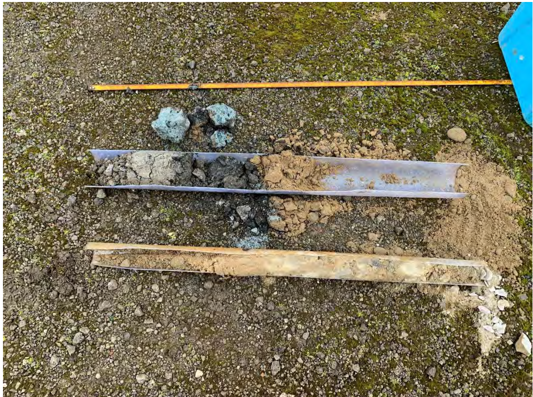
Photograph 8: Materials recovered from WS04, 0.0 – 2.0mbgl.
