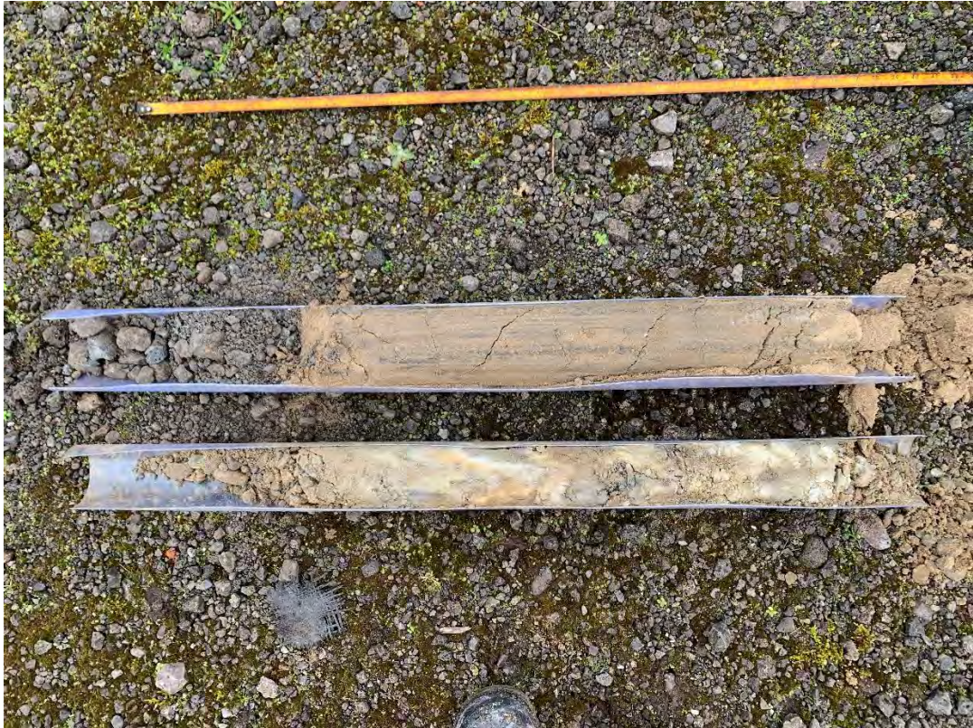
Photograph 7: Materials recovered from WS03, 0.0 – 2.0mbgl.
