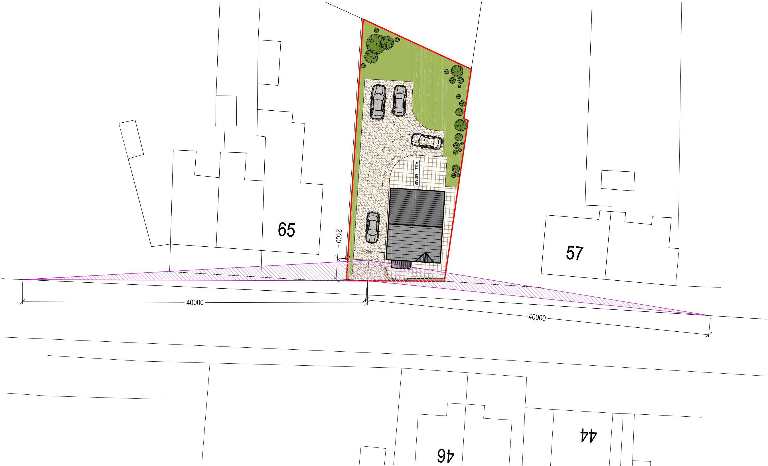
PROPOSED SITE PLAN - Visibility splays Scale 1:250
