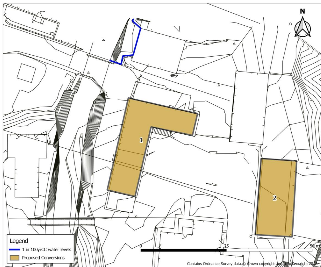
Figure 6 1% AEP+CC out of bank water levels as shown for the blockage scenario (projected to site contour data)
