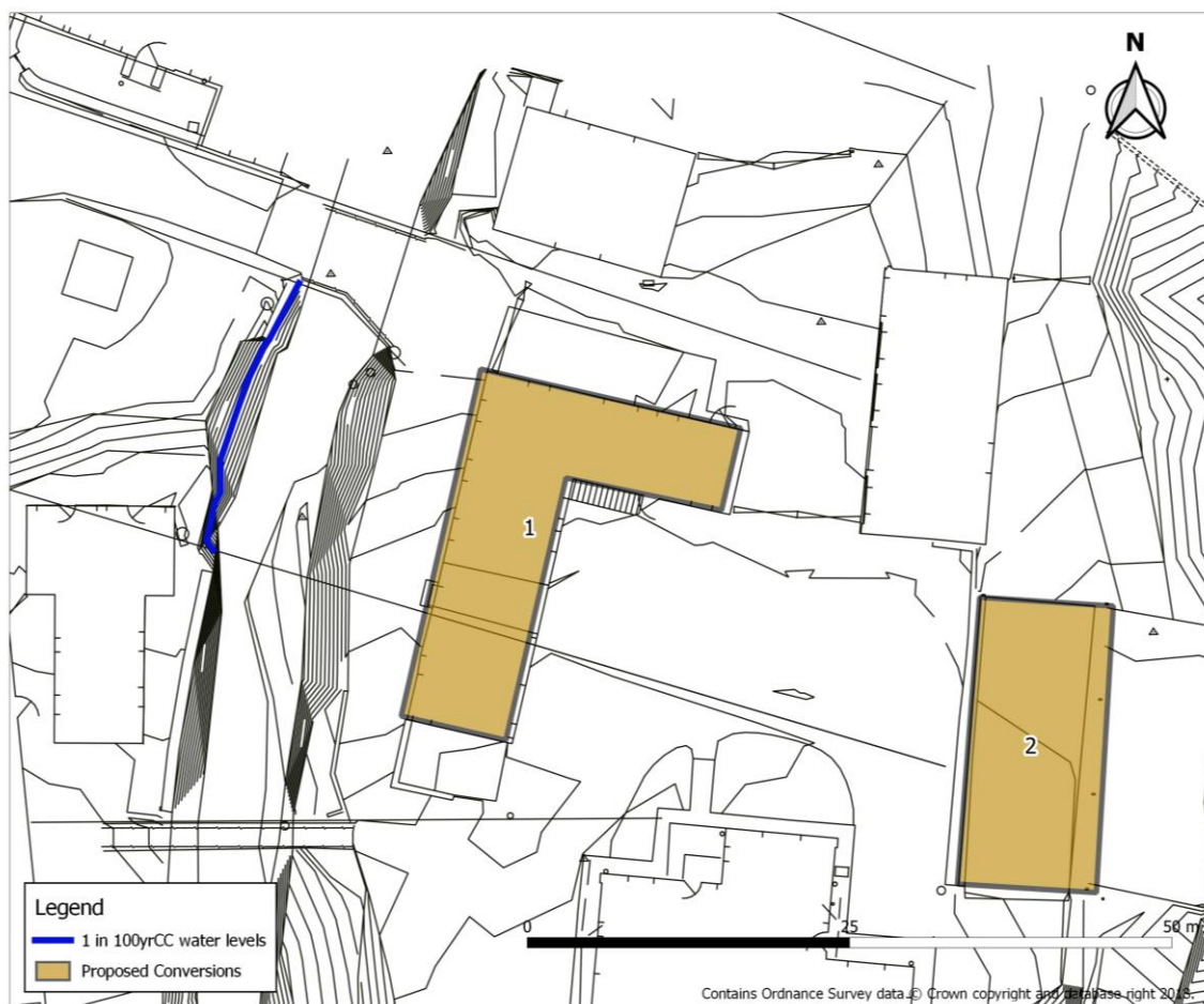
Figure 4 1% AEP+CC modelled out of bank flood levels (as projected from the 1D model to site contour data)
