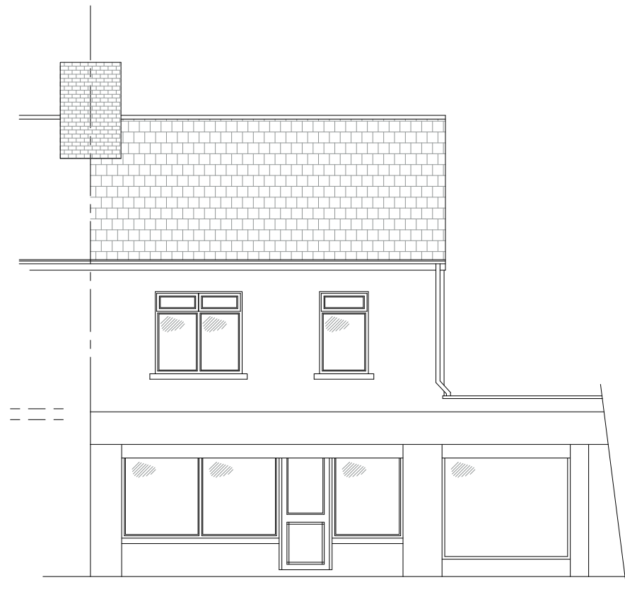
EXISTING FRONT ELEVATION scale 1:100
