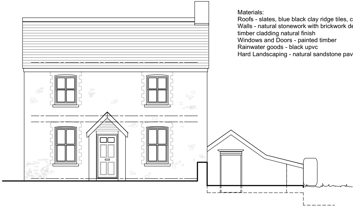
Front (south east) Elevation
