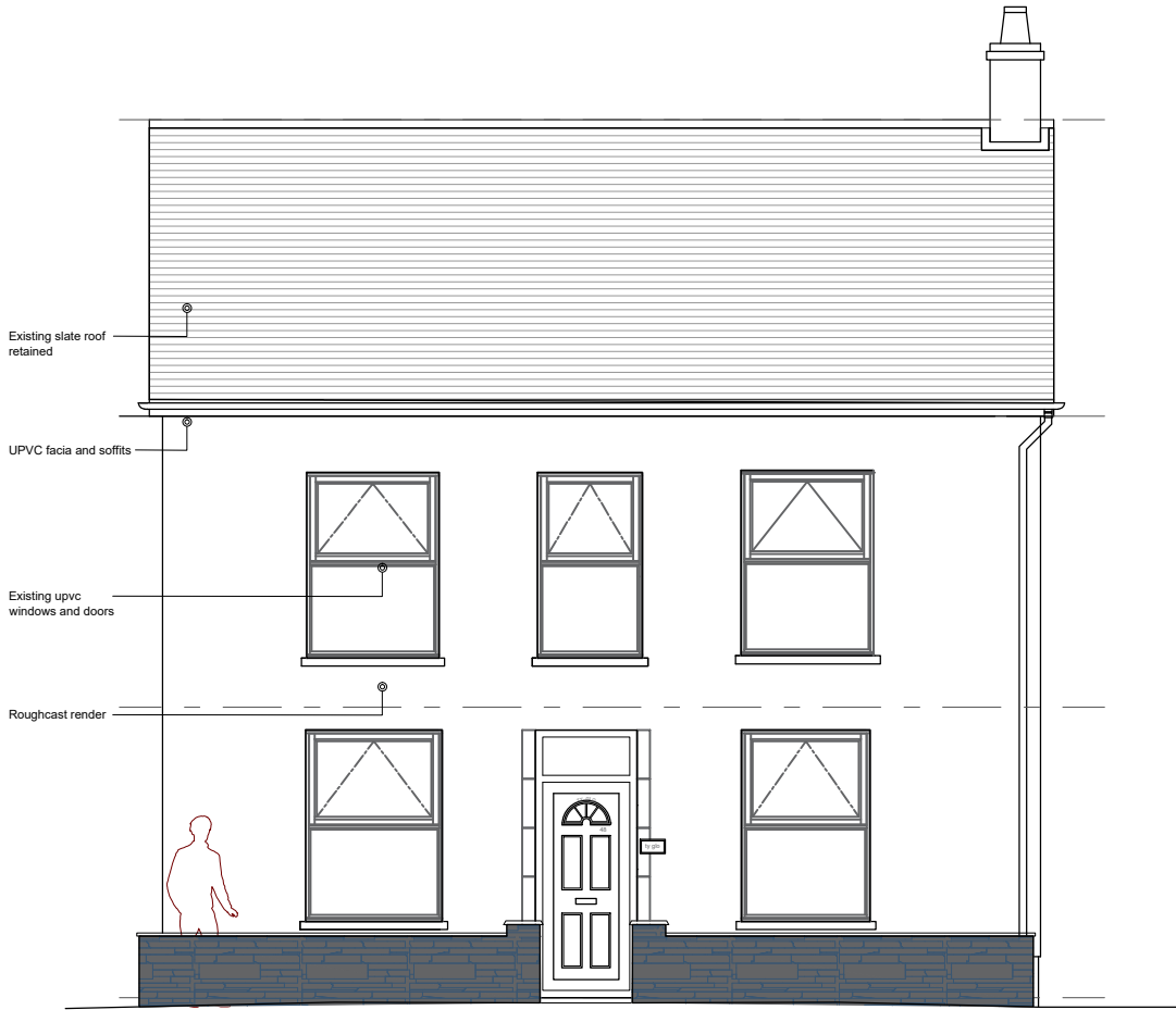
Existing Front Elevation
