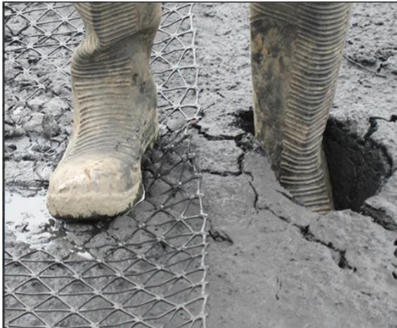
With Tensar Layer / Without Tensar layer
