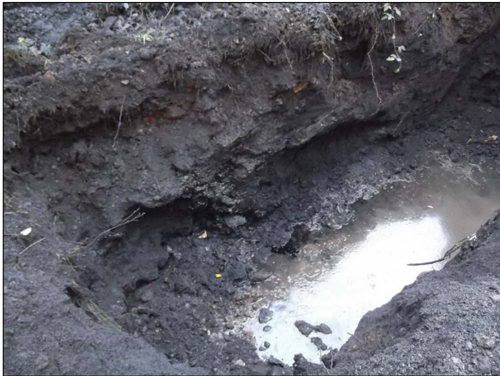
Photograph 7 – Observations of groundwater and free product in slit trench
