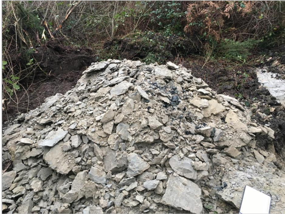
Photograph 17: Arisings from TP10 - possible china clay used in refinery processes and disposed of in the Tip
