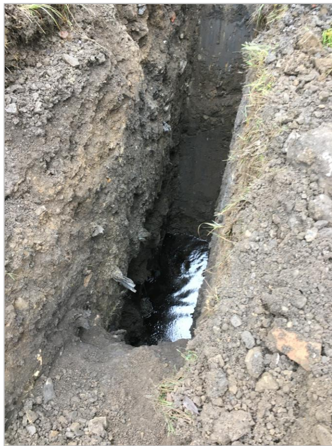
Photograph 6: TP03 free product on groundwater
