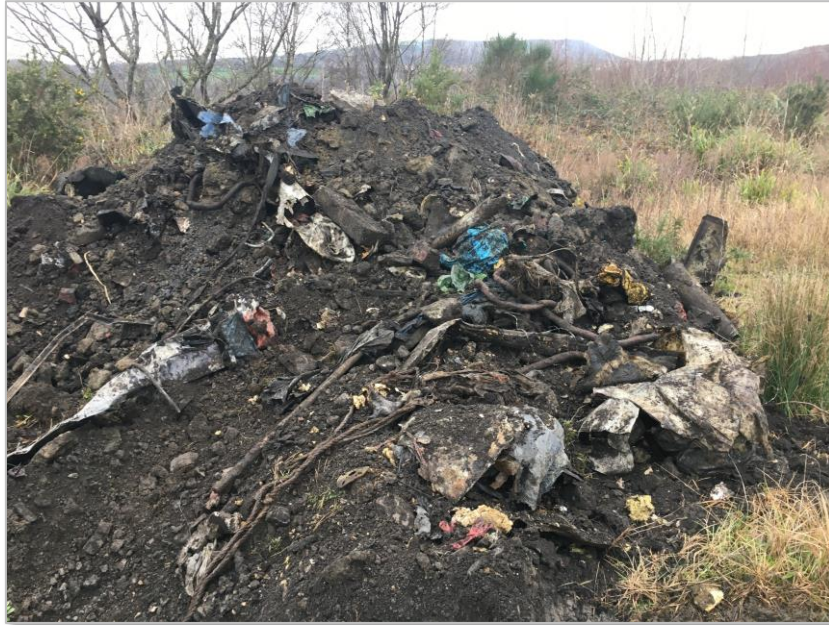
Photograph 3: Arisings from TP02 including plastic, fire hoses cables and pipes
