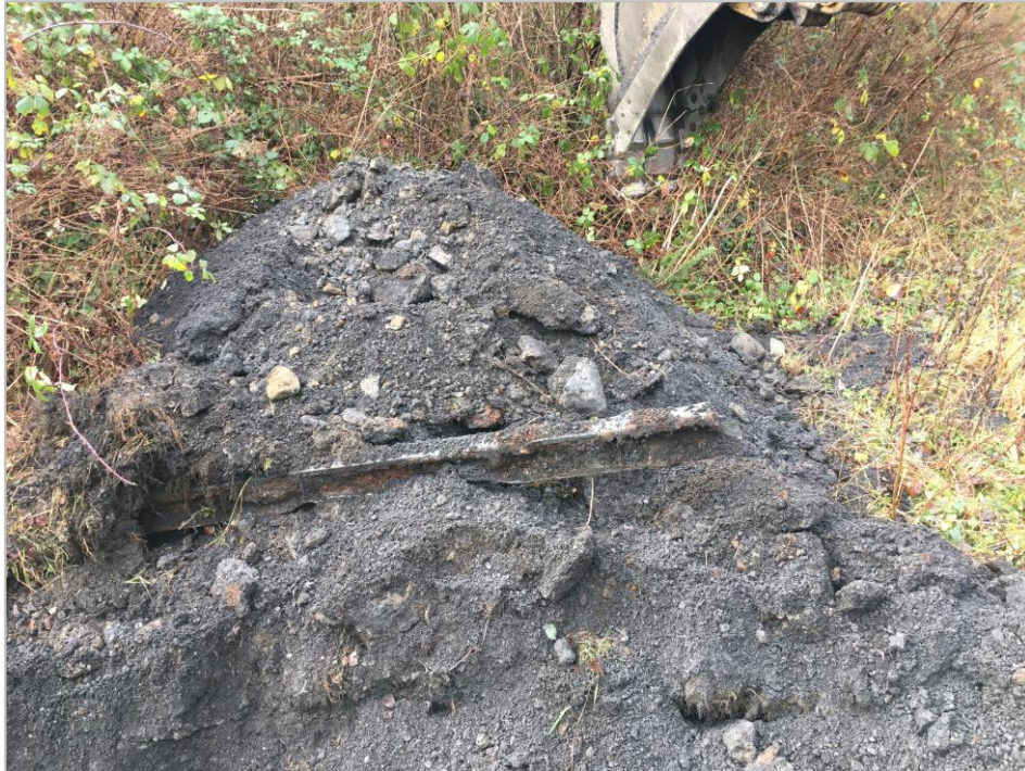
Photograph 15: Arisings from TP08 with metal waste visible
