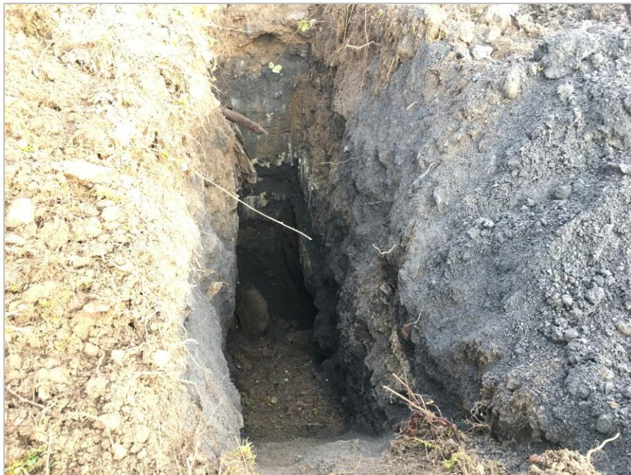
Photograph 14: TP07 excavation - predominantly ash
