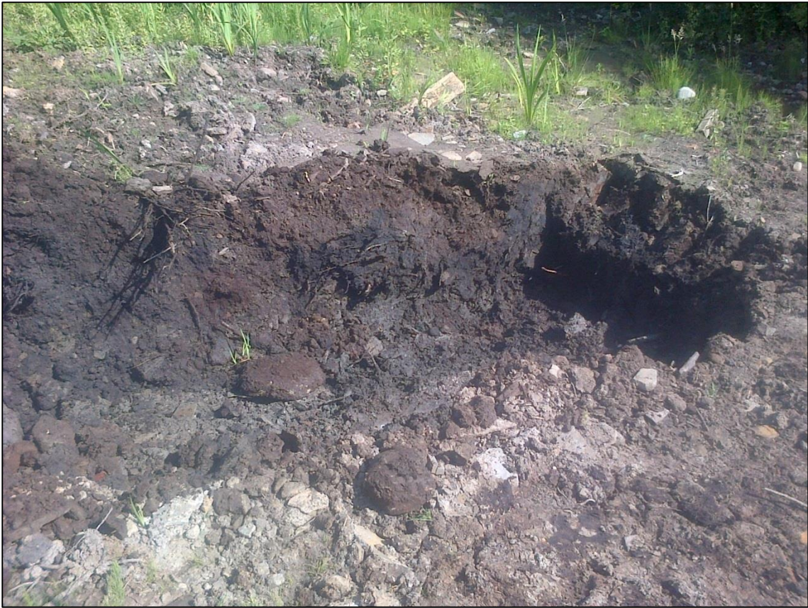
Photograph 1 IP1739 – Black peat in excavation with no evidence of free product.
