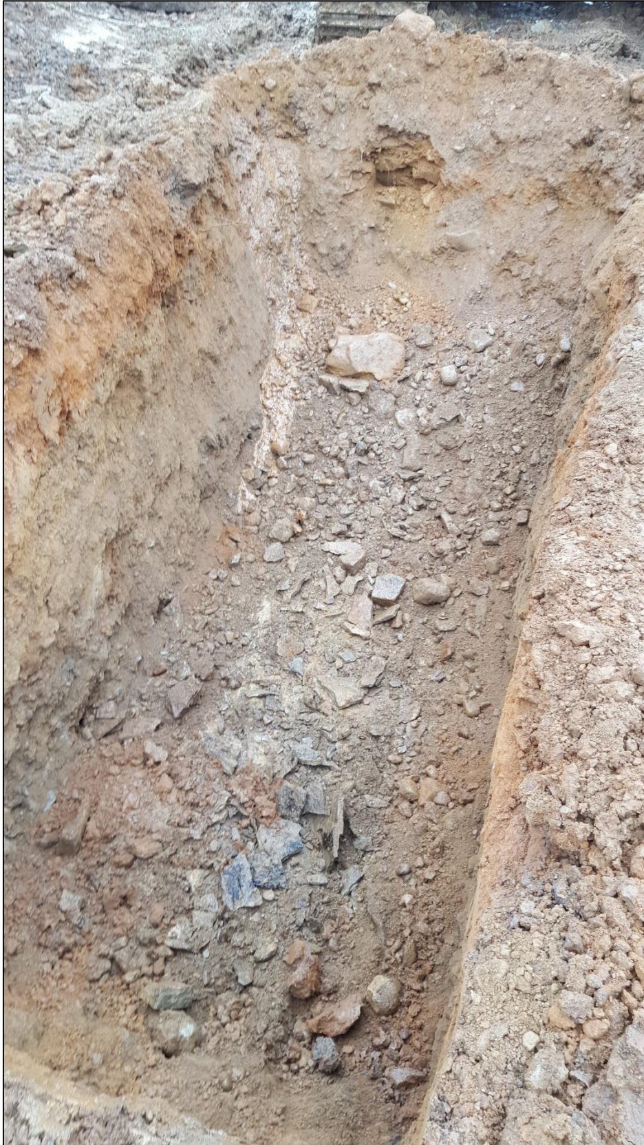
Photograph 4 TPE2742 – Minor pockets of hydrocarbon staining on weathered bedrock gravel at base of trial pit
