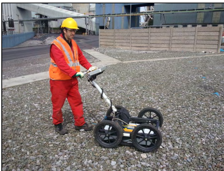
Plate 3 – MALA RAMAC 250MHz GPR cart system (library photograph)
