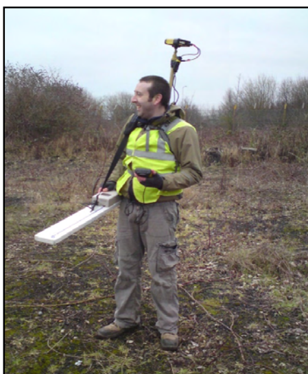
Plate 2 - Geophex GEM-2 with Trimble DGPS positioning (library picture)
