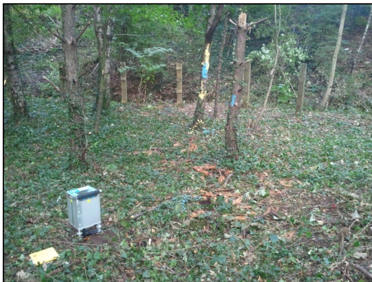
Plate 4 – Scintrex CG-5 gravity meter being used in Shaft 2 area
