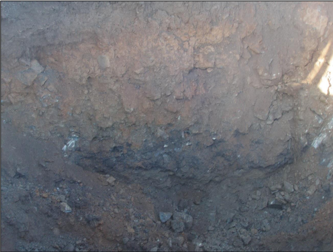
NSE31A Face of excavation. No visual or olfactory evidence of contamination
