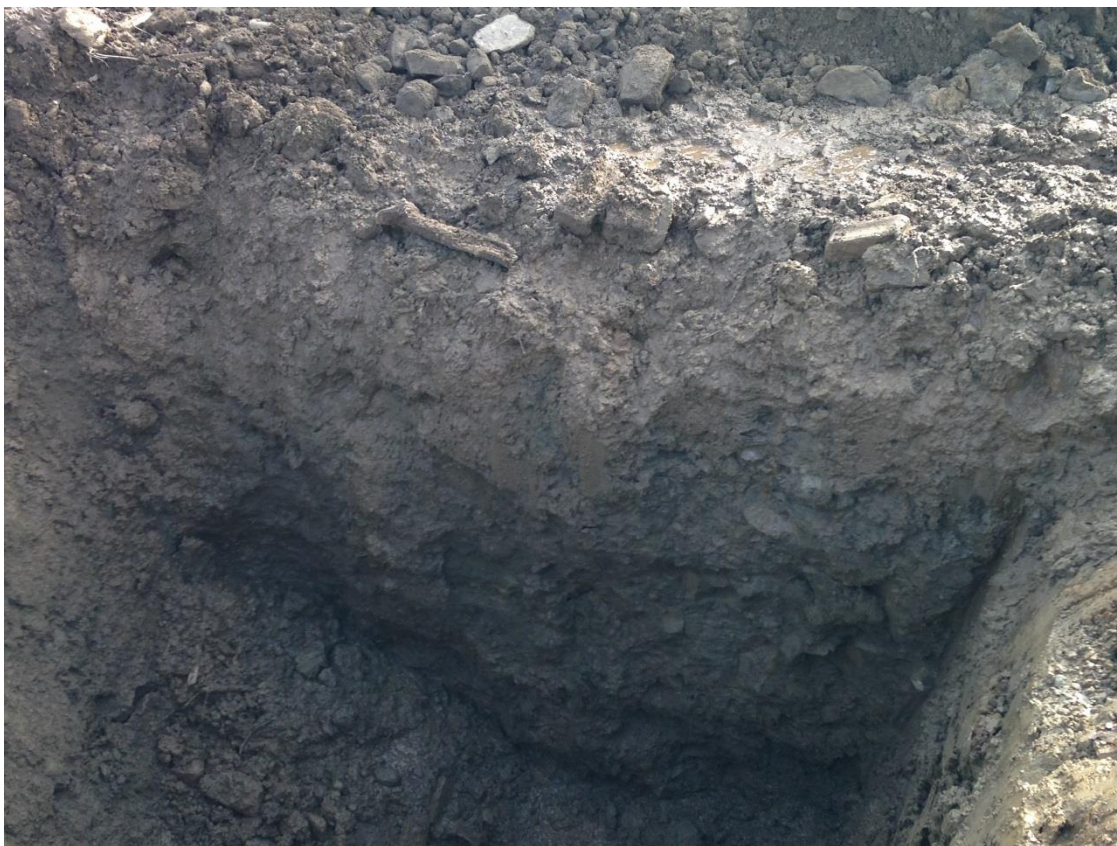
Photograph 1 NSW142 – investigation in to observed thick oily sludge during ground investigation. Material assigned VO score of 1,2
