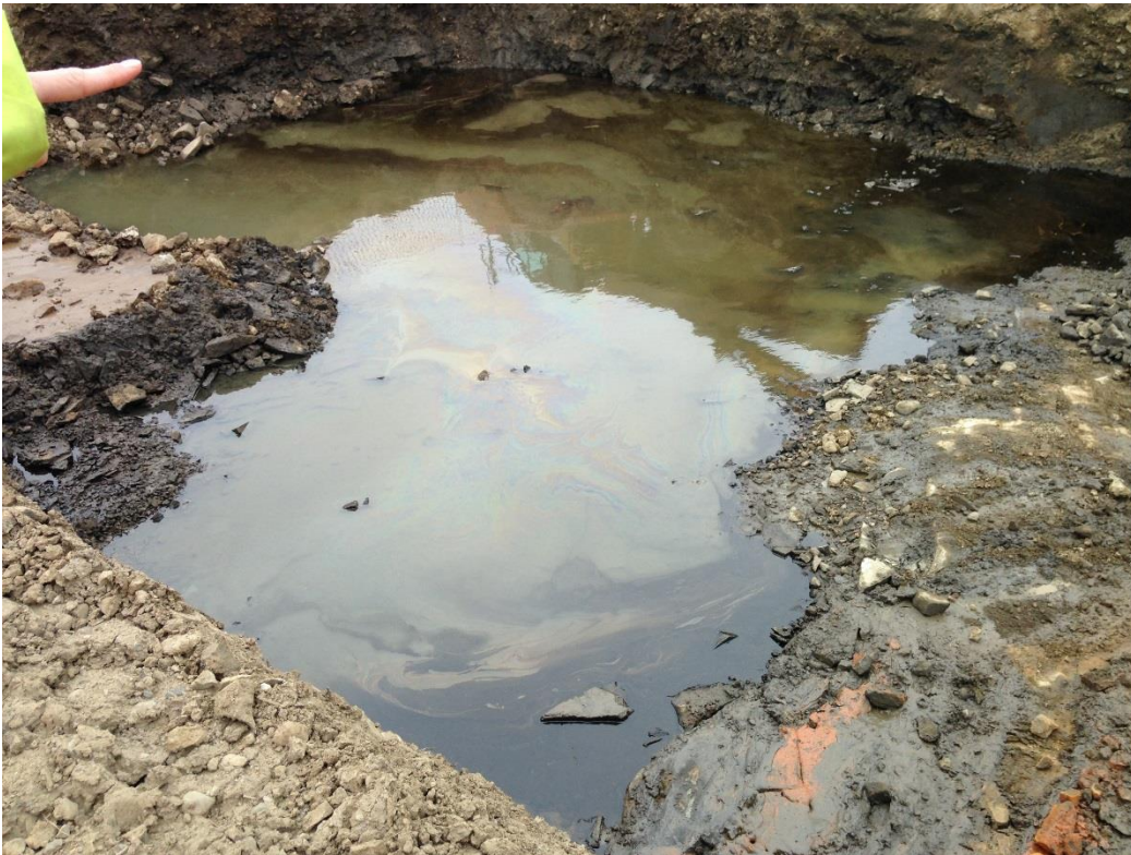
Photograph 8 NSW910, NSW942, NSW943 – free product on groundwater in the base of a combined excavation to investigate thick oily sheens and assigned scores of 5 in the area of NSW910, NSW942 and NSW943
