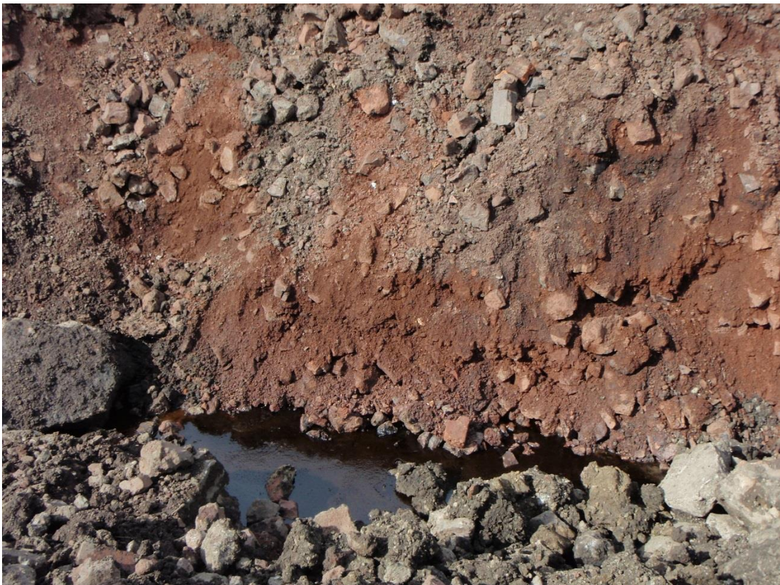
Photograph 10: Localised areas of free product within shallow Made Ground
