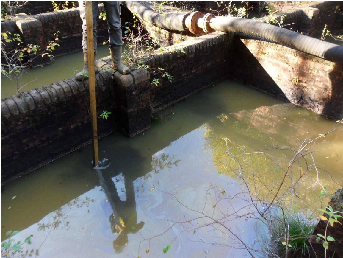
3) Agitation of basal silts to observe entrained product. Only sheens observed.
