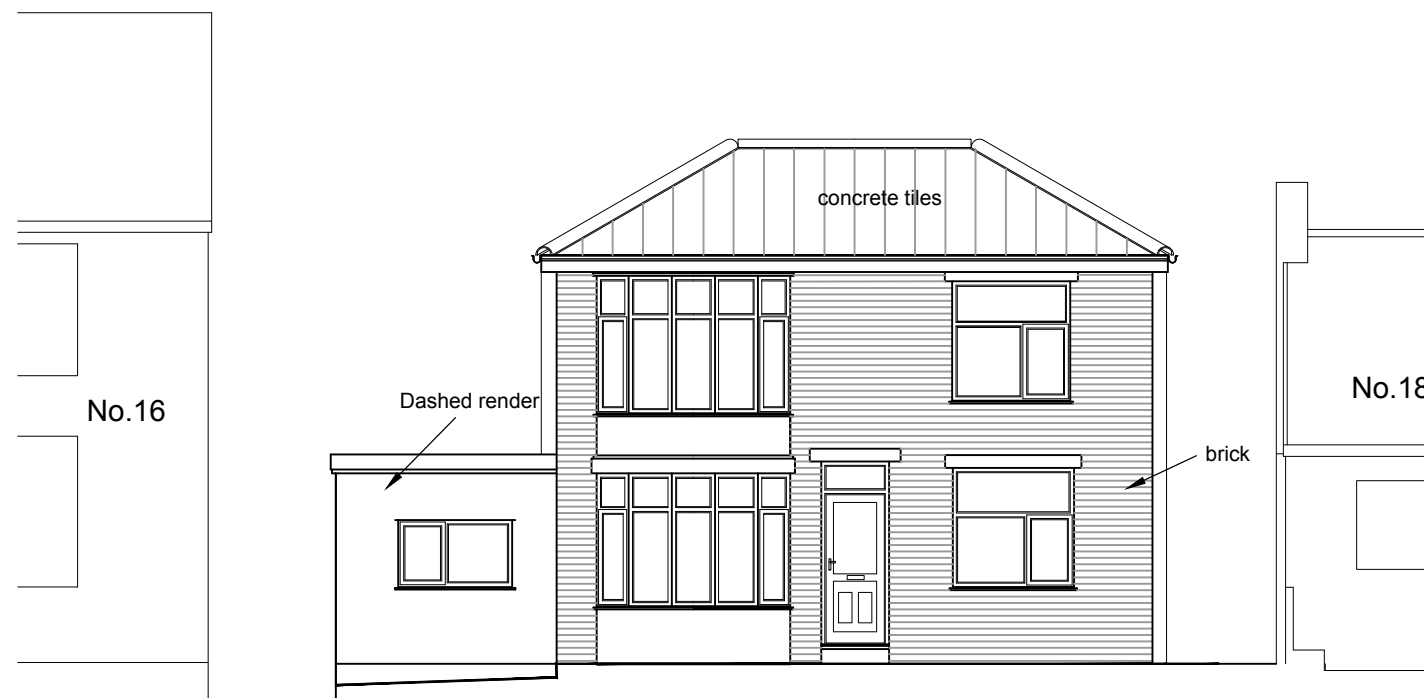
EXISTING FRONT ELEVATION
