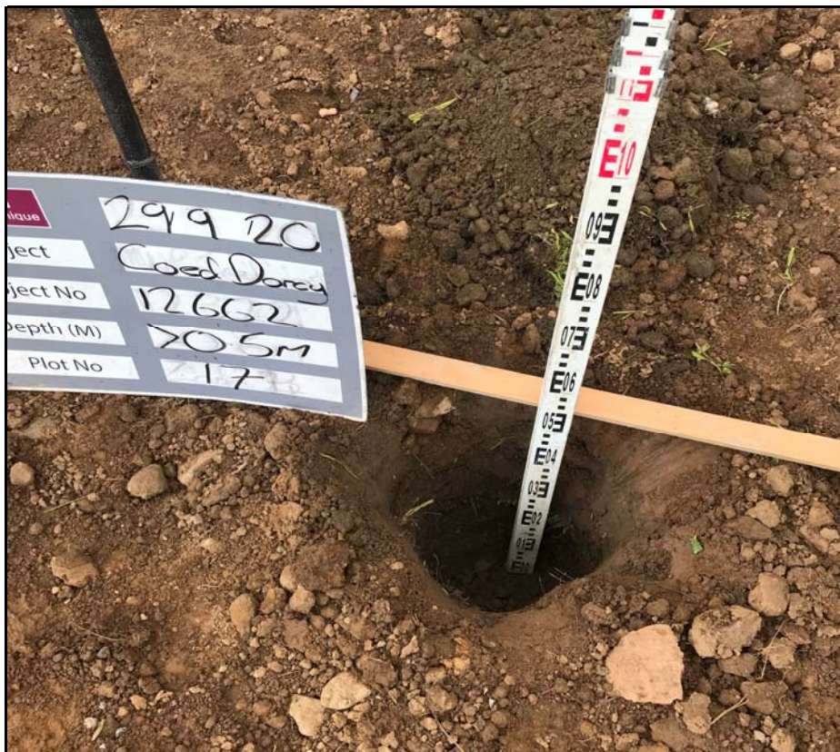
Plot 17 Excavation Trial Pit
