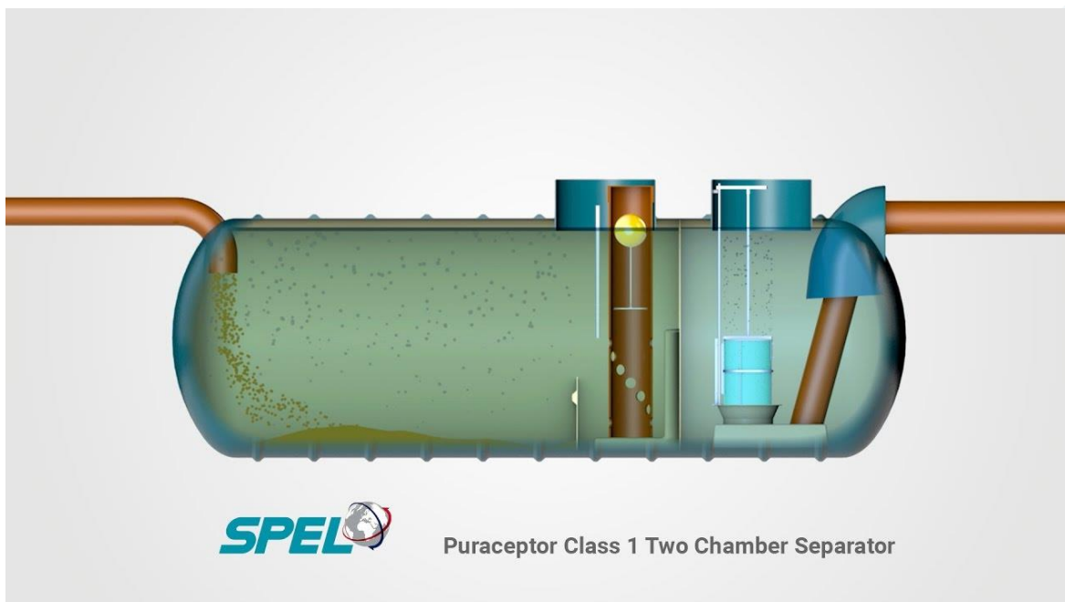
Figure 3-4 Example of a class 1 full retention separator (SPEL Products)
