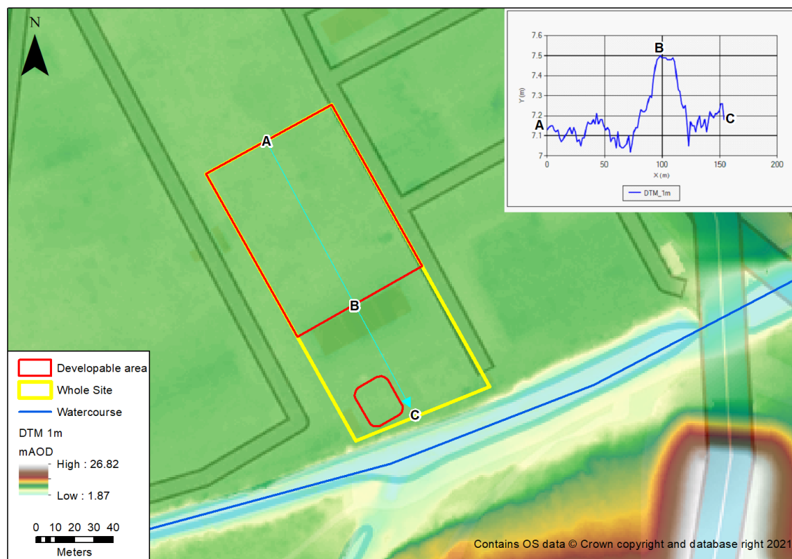
Figure 1-2 Site topography using NRW 1m LiDAR
