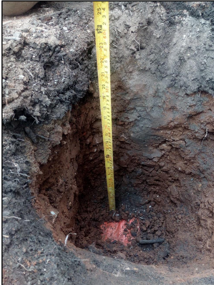
Plate 01. Capping Soils and Barrier at >600mm bgl.
