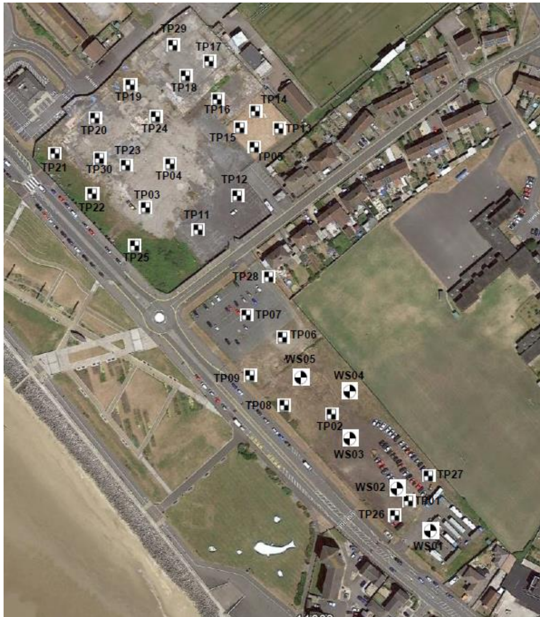
Figure 2.1: Terra Firma Exploratory Hole Layout
