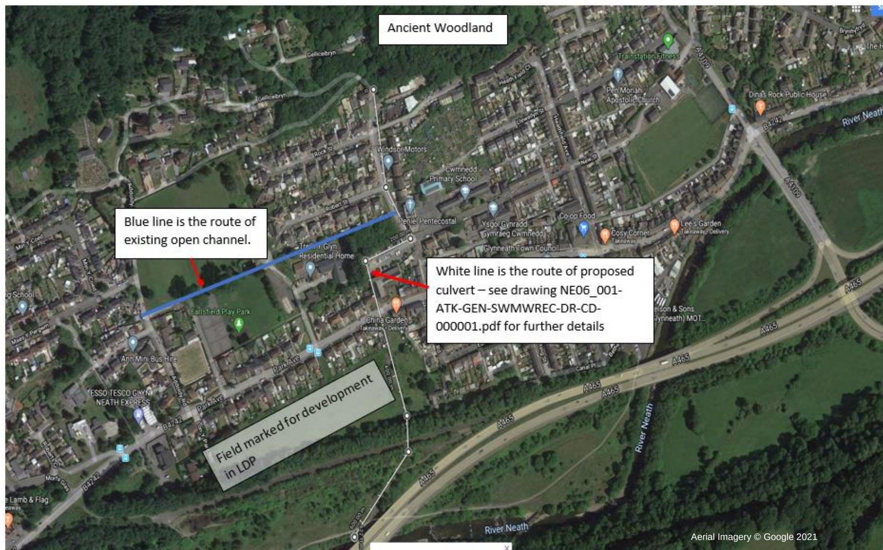
Figure 1-1 – Phase 1: Culvert diversion from Gelliceibryn Brook
