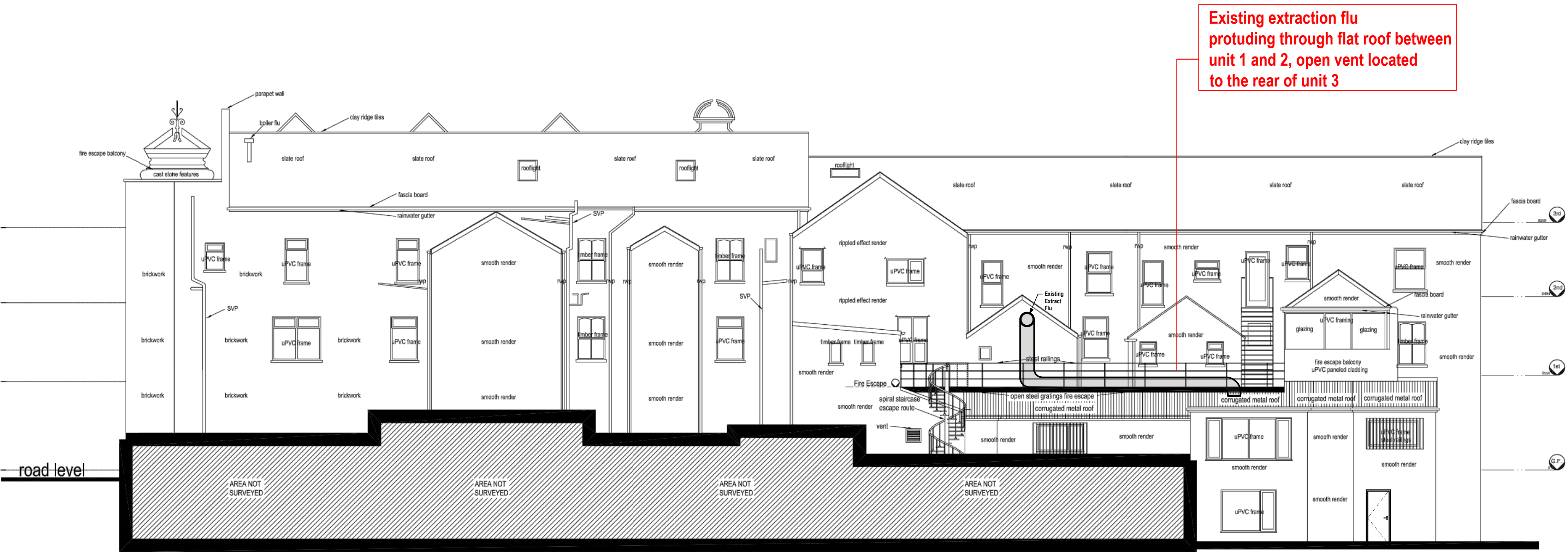
NORTH-WEST ELEVATION : as existing
