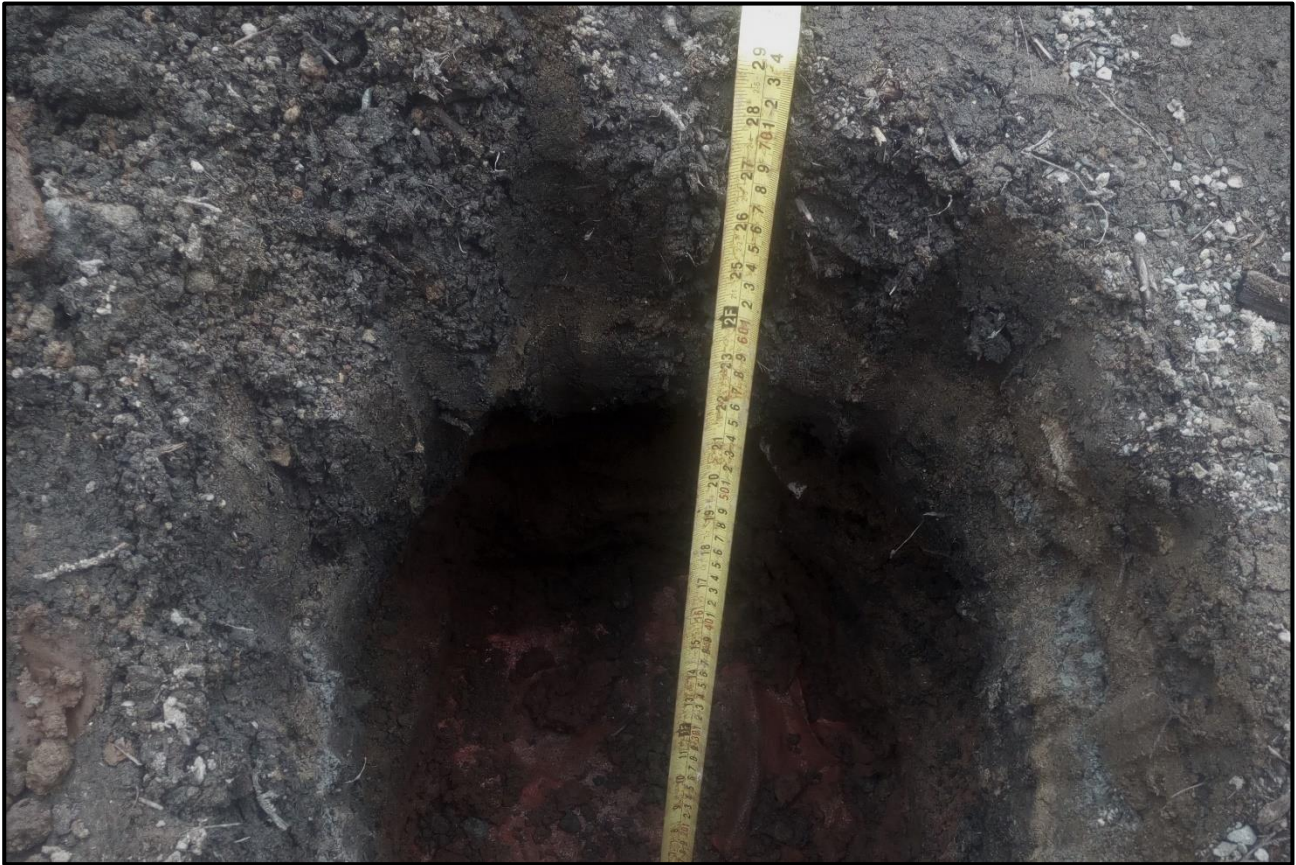
Plate 01. Capping Soils and Barrier at >600mm bgl.
