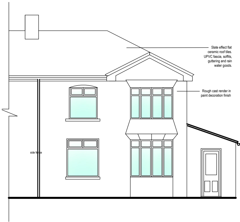
Existing Front Elevation Scale 1:100 @A3 (Retained)
