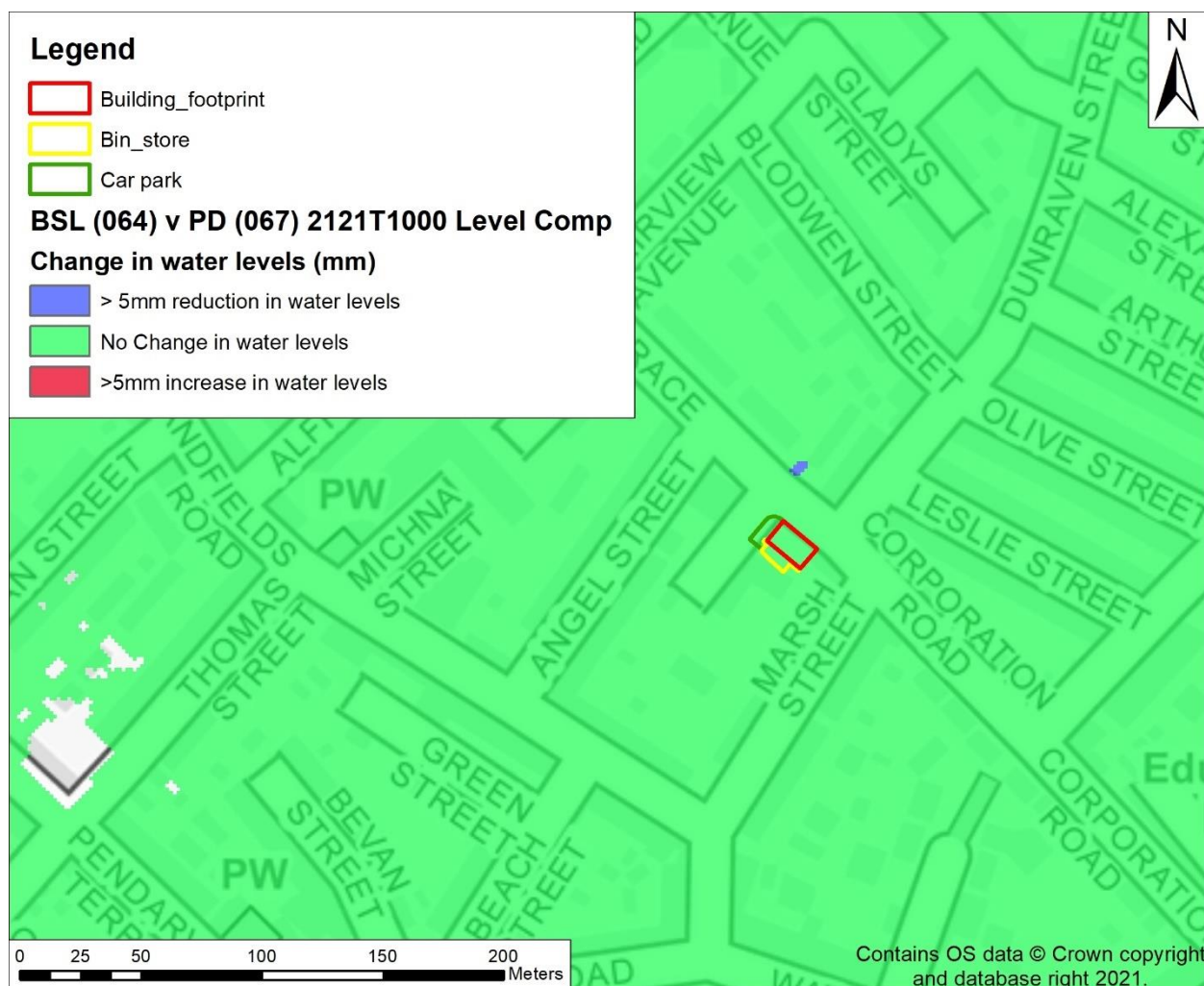
Figure 4-13: 2121 0.1% AEP tidal event level grid comparison
