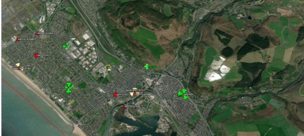
Figure 1 – Coverage Plots showing the required area to be covered showing the best location from a coverage perspective – needs to be as close as possible to green marker.
