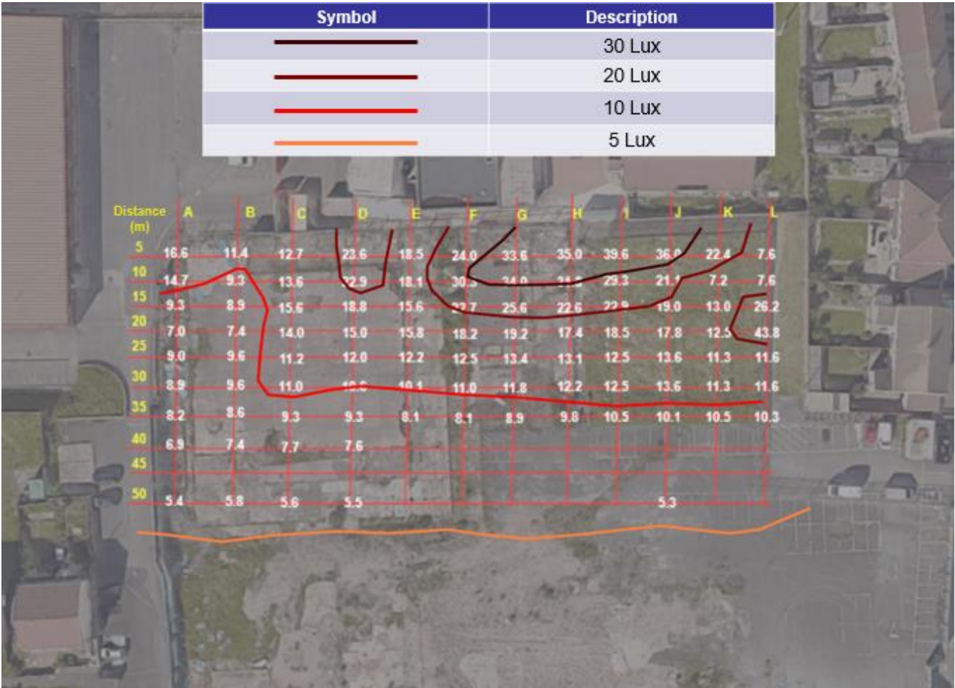
Figure 3-4 – Pre-LED Floodlighting Contour Lux Lines on Proposed Residential Development Transect
