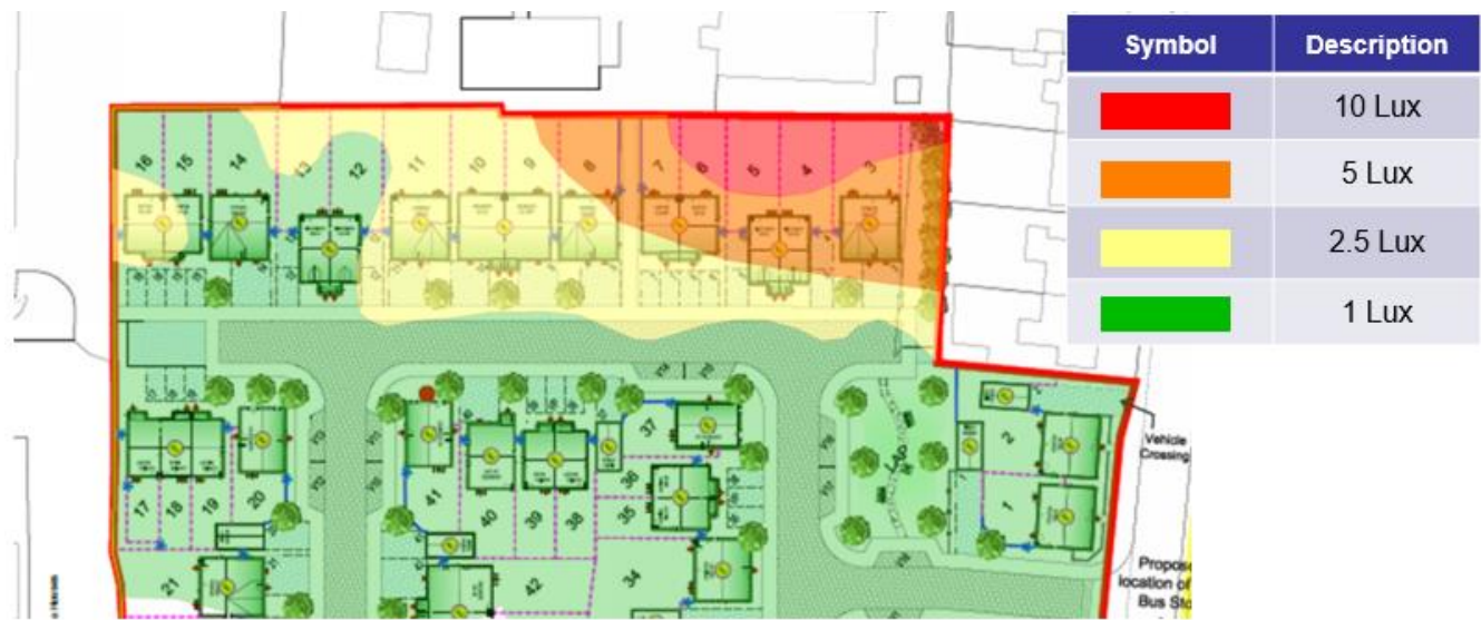
Figure 3-10 – Post-LED Contour Lux Plot on Proposed Residential Development
