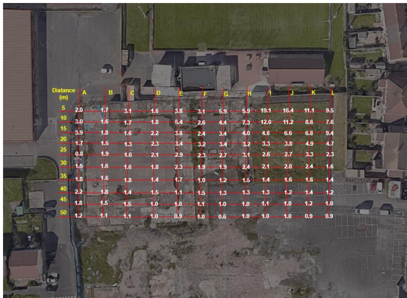
Figure 3-8 - Post-LED Floodlighting Lux Levels on Proposed Residential Light Monitoring Transect
