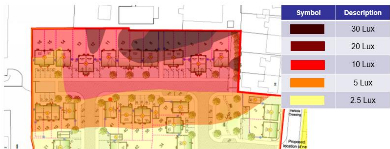
Figure 3-5 – Pre-LED Contour Lux Plot on Proposed Residential Development
