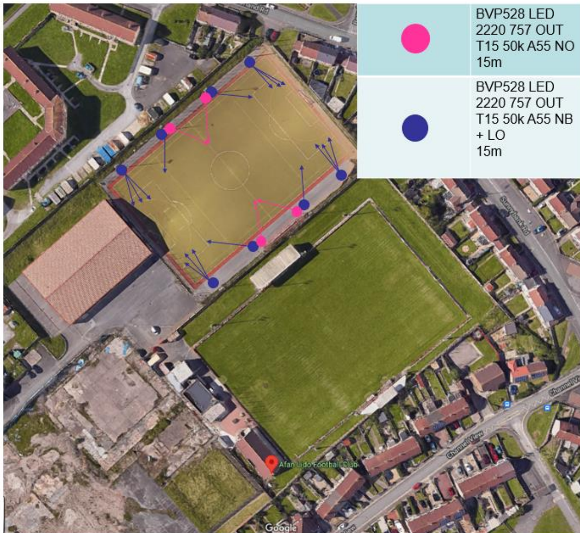
Figure 8 – Potential Lighting Design for “Astro Turf” Pitch using 350lx Football Pitch Lighting Design.
