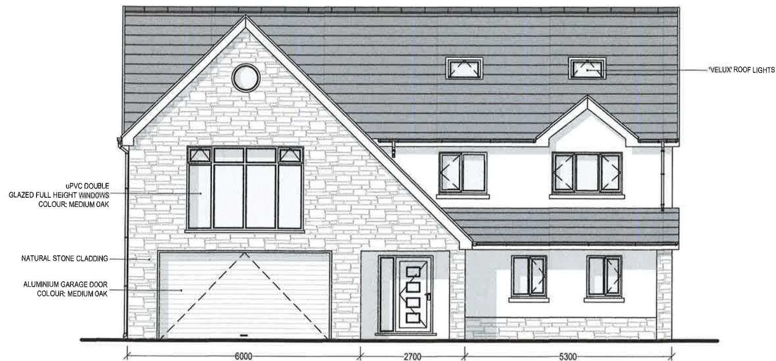
PROPOSED FRONT ELEVATION Scale 1:100
