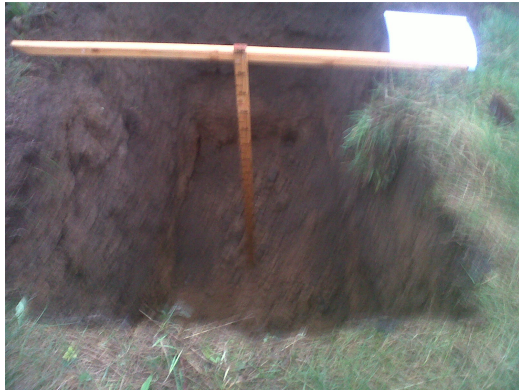
Photograph shows excavated Trial Pit 1 with 1600mm long timber measuring tool resting on base and top edges.
