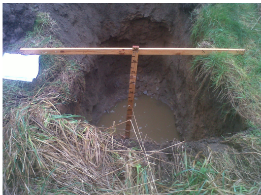
Photograph show Trial Pit 2 after 60mins with approximately 200mm of water remaining.
