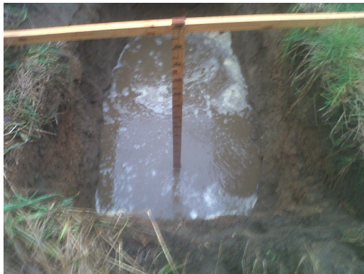
Photograph shows Trial Pit 2 filled with approximately 400mm of water.
