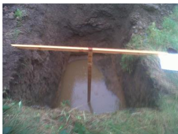
Photograph shows Trial Pit 1 after 60mins with approximately 200mm of water remaining.
