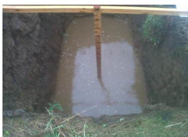
Photograph shows Trial Pit 1 filled with 400mm of water.
