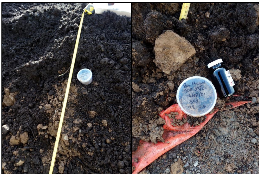
Plate 02 & 03. Capping Soils 23/24 & No Dig Barrier 23/24
