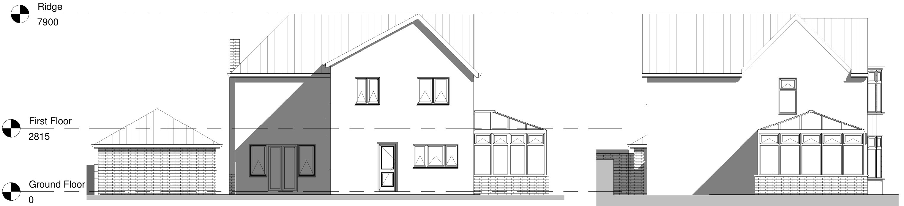
EXISTING REAR ELEVATION - EAST SCALE 1:100
