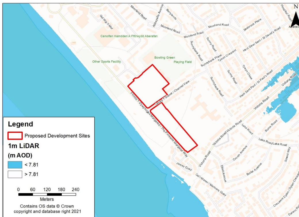
Figure 4-1: Ground levels compared to the extreme sea level prediction for the 0.1% AEP event plus 100 years of climate change (7.81m AOD)
