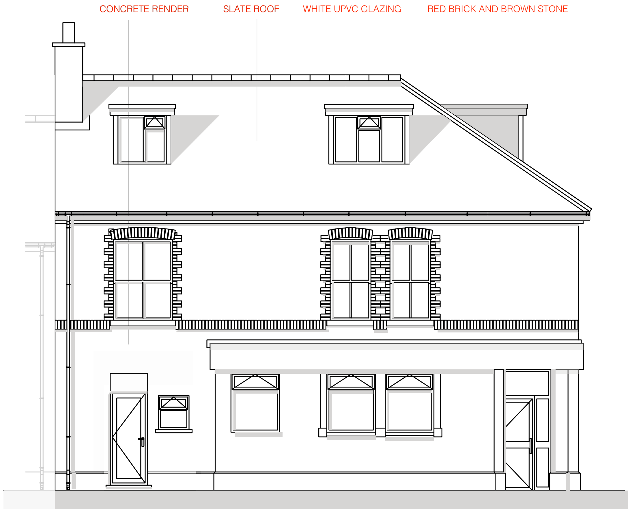
FRONT ELEVATION NORTH WEST 1.50
