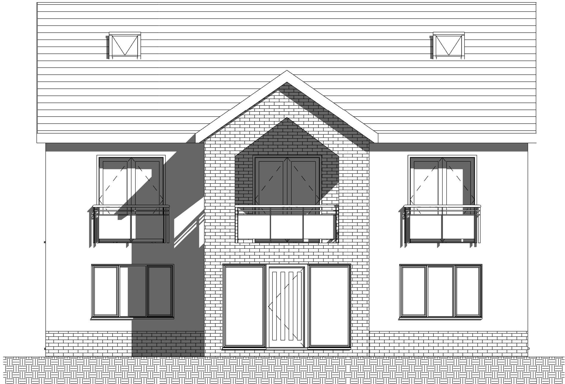
Front Elevation Scale 1:50
