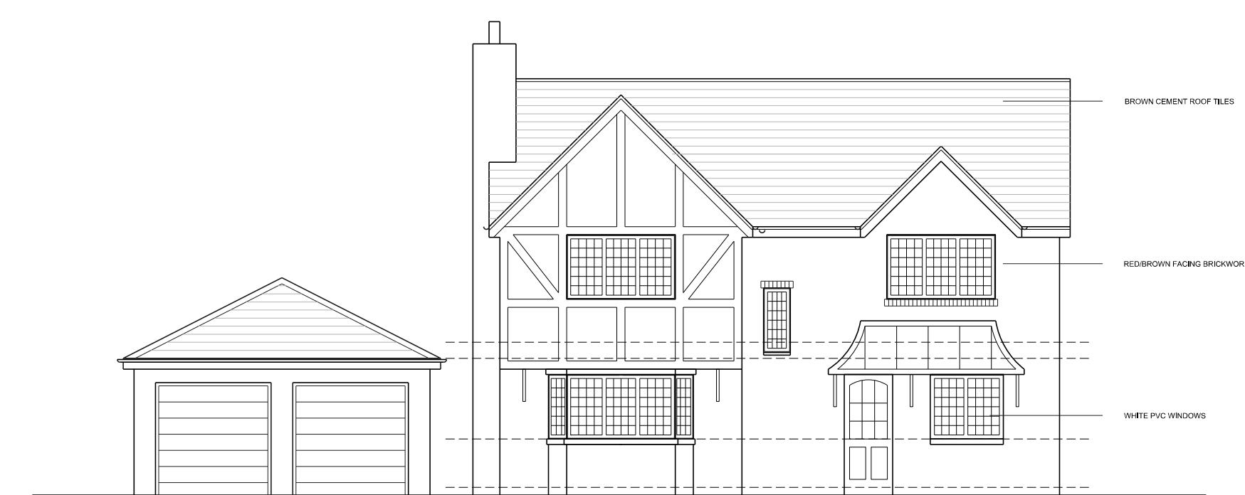
EXISTING FRONT ELEVATION SCALE 1:100
