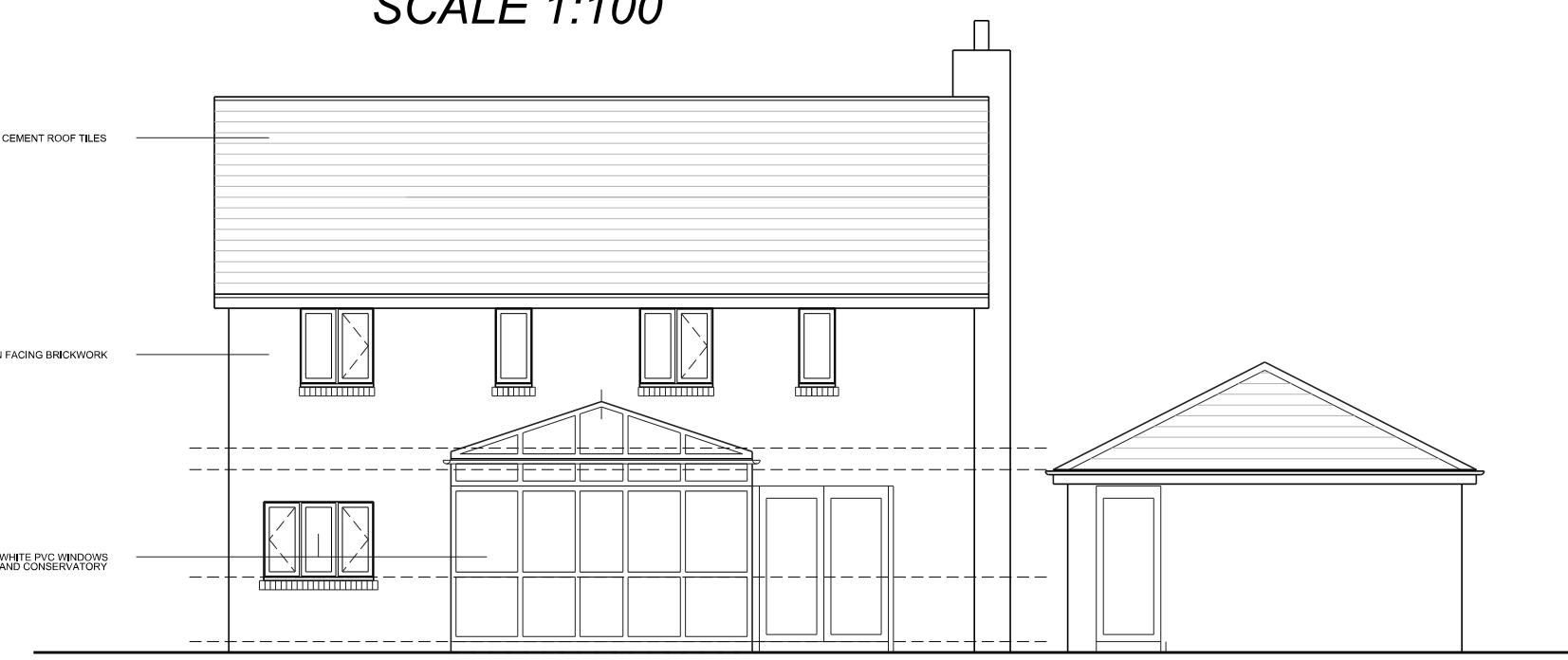
EXISTING REAR ELEVATION SCALE 1:100
