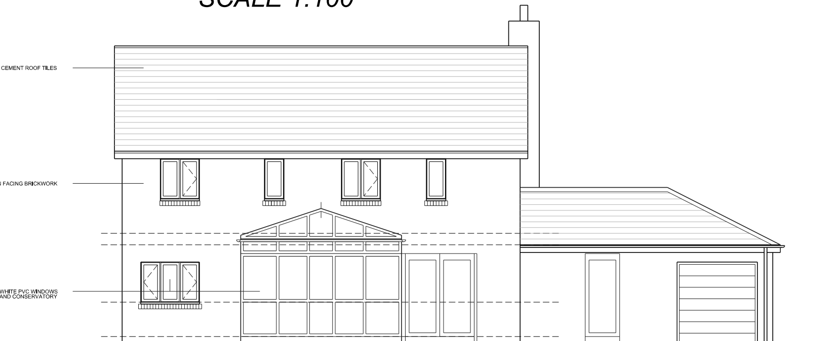
PROPOSED REAR ELEVATION SCALE 1:100
