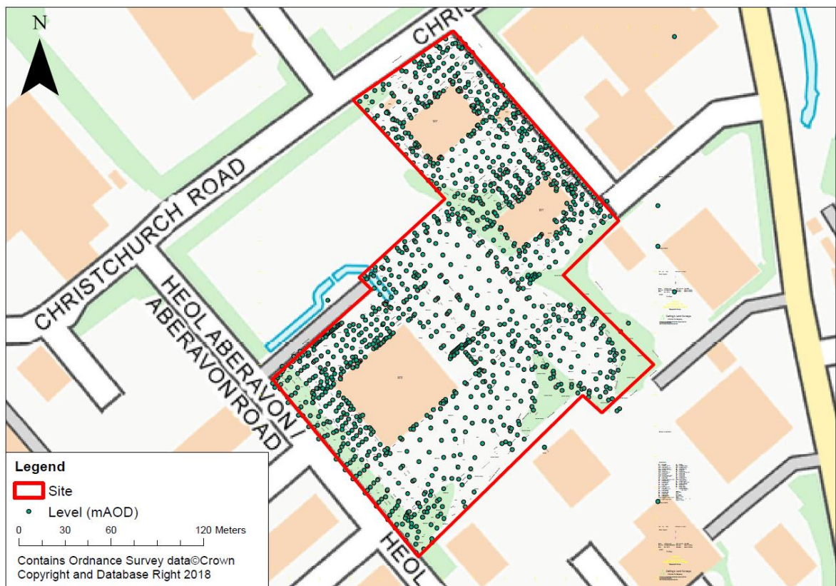
Figure 2-4. Topographical survey extent
