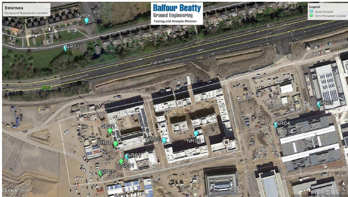
Figure 2. BBGE Noise and Vibration Monitoring Locations (January-April 2016)
