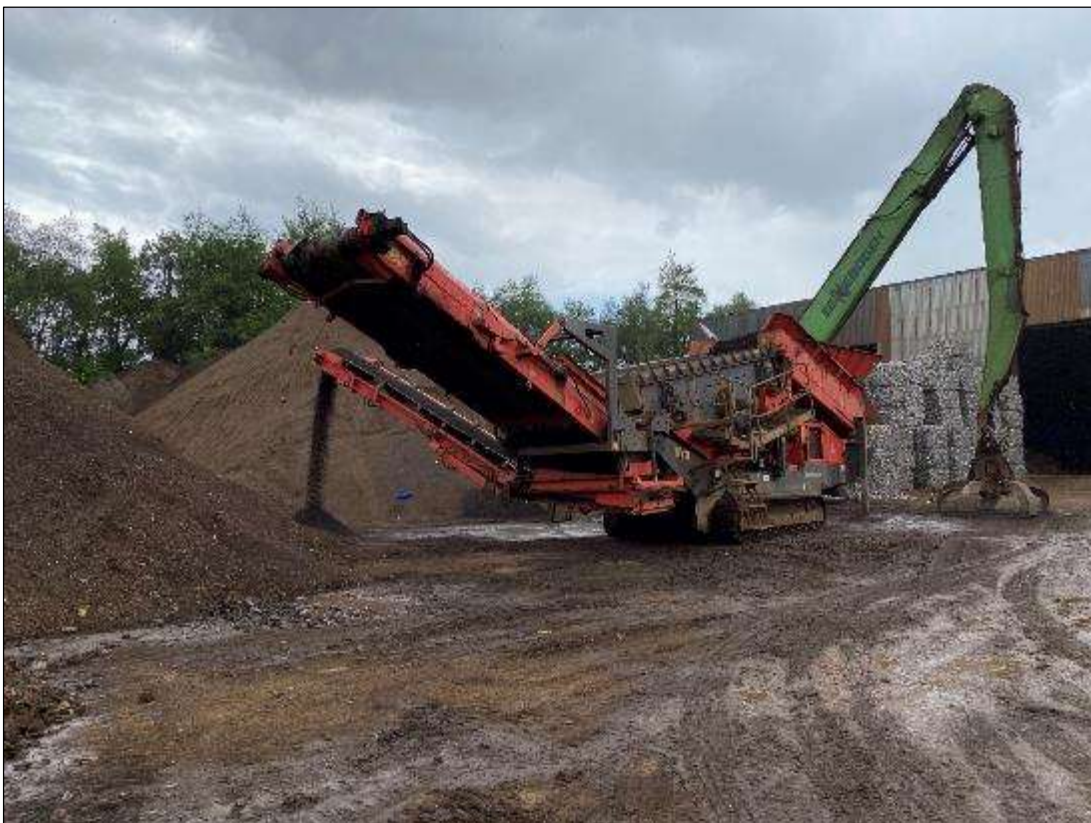
PHOTO 'H': Screening plant in central part of the site. Incinerated scrap metal and aggregates are processed and stockpiled adjacent to it.
