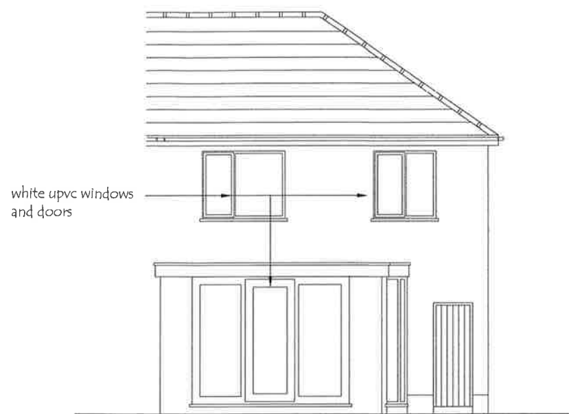
Existing Rear Elevation
