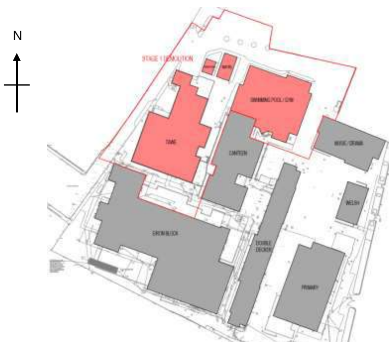
Figure 1-1. Existing Site Plan Showing Extent of Demolition
