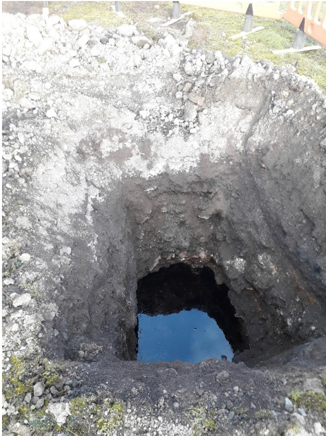
Plate 5: TP203A with free phase LNAPL contamination. photo taken on 04/12/2019
