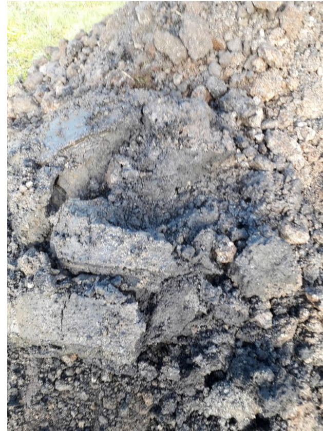
Plate 6: Hydrocarbon impacted arisings from TP203A. photo taken on 04/12/2019
