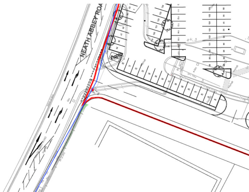
Figure 5.1 – Indicative Site Access with Right Turn Lane
