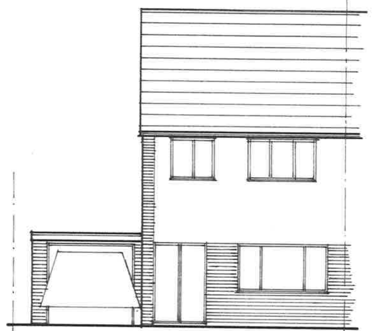
Existing Front Elevation
